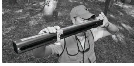
The Jim-Gem Wheeler Pentaprism Caliper is used as a precision optical-prism device to accurately measure tree diameters at DBH, or any height point from any clear, convenient sight position. The caliper contains two pentaprisms, one fixed and one movable, which are mounted in a tubular metal frame permitting simultaneous viewing along parallel lines of sight to the tree being measured. The caliper is constructed to measure stems from 3" to 24" (7cm to 62cm), and is accurate to 1/10 inch (±2 mm).
