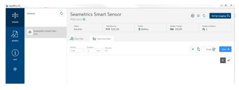
To start real-time readings click Start, readings default to table view. To switch to Real-time graphing view click the graph icon
