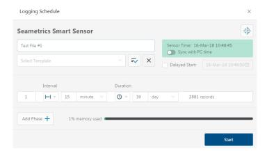
Click to switch between interval and continuous data recording (supported sensors only) Select your continuous rate from the drop down box (on the right).
