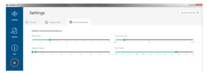
Simply drag the Address Range slider higher up to increase the maximum Modbus address scanned. If you've scanned all the way up through address 255 and still have no connection click Troubleshooting for further troubleshooting or contact Seametrics Tech Support for assistance.
