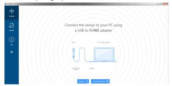
If your cable and sensor were not connected before opening Aqua4Plus 2.0 simply connect and click Rescan. While scanning is active you'll see a green dot flash in the upper right corner of the program. Scanning is complete when this dot stops flashing.
