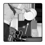
2) Open the foam tank valve and turn the dial clockwise to the desired foam rate.
