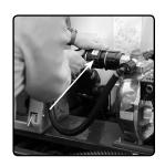
**3)** Attach suction hose from Quick-Fill™ draft kit to suction part of pump. Ensure water is present in the bottom of the pump housing to allow unit to self prime.
