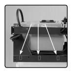
**2)** Install two d-ring tie-downs on each side of the frame using the supplied nuts and bolts.
