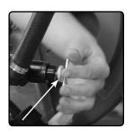
**4)** Before starting your engine, make sure the drain plug and prime plug are tightened securely and properly holding the seal O-rings in place.
