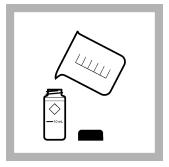
3. Prepare the sample: Fill a sample cell to the 10-mL mark with sample or diluted sample. Refer to Sample dilution on page 2.
