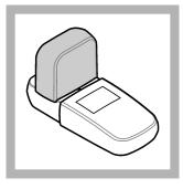
**12.** Install the instrument cap over the cell holder.
