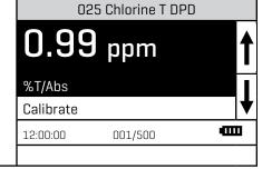
9. Press ENTER to select Calibrate. A reverse font (light background with dark characters) will appear to indicate that the reading can be adjusted.
