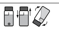
Immediately insert tube into chamber. Close lid. Select Scan Sample. Record result as Free Chlorine.
