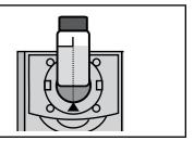
6. Remove tube from colorimeter. Add one \*Chlorine DPD #1 Instrument Grade Tablet (6903A).
