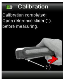
**Note:** An error will be displayed if the white reference slider was not in the correct position for calibration. If this occurs, close the slider and repeat the calibration process. After recalibration this message continues, refer to Troubleshooting in the Appendices.
