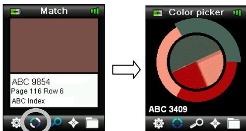
3. Color descriptions for each color can be displayed by pressing on the up or down sides of the **Navigation** control. The selected color is highlighted around the circle.
