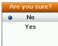
3. Highlighting **Yes** on the screen and press the **Enter** button. All records are now deleted from the instrument.
