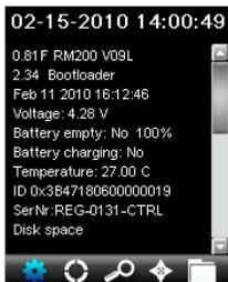
Version information for the fan decks currently installed in the instrument can be found at the end of the Product Info screen.
