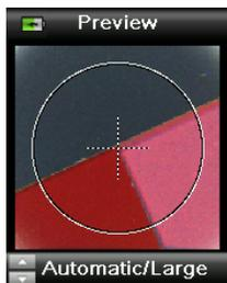
The initial color displayed in the Match window is the average color across the measurement area. Once CAPSURE detects a sample containing more than one color, the Color Picker icon in the function bar begins rotating and an audible tone is heard. The screen then automatically advances to the Color Picker function. Individual colors are selected from this screen.
