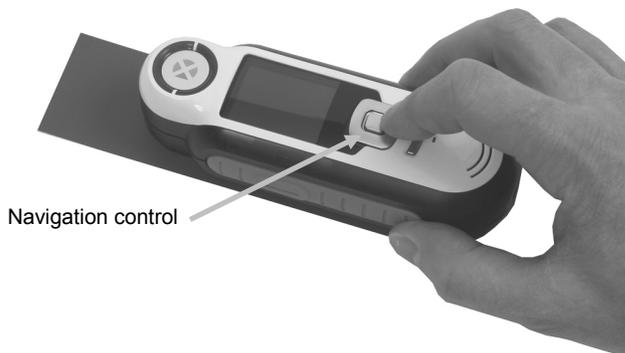
Depending on the fan deck selected, additional information associated to the color can be displayed and selected using the Navigation control.
