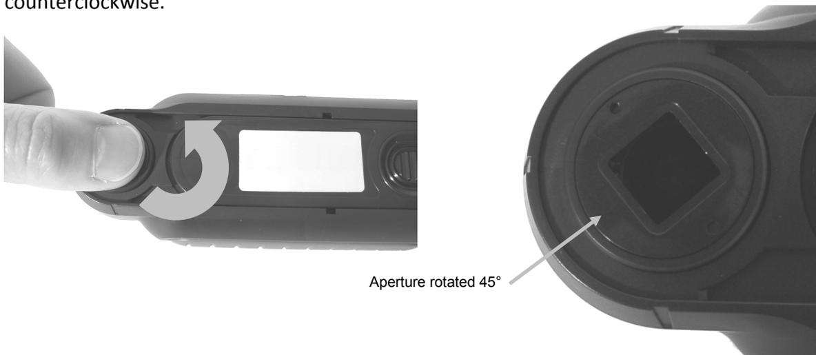
2. Remove the aperture from the optics housing and set aside.
