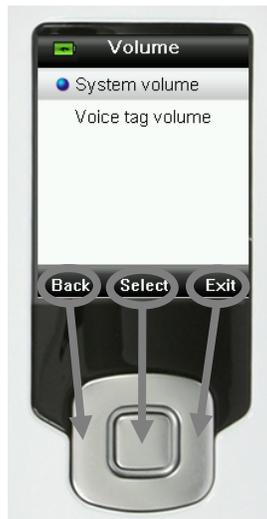
Screens that contain images of “arrows” indicate that the Up and Down sides of the Navigation control are used to adjust or page-through options and colors.
