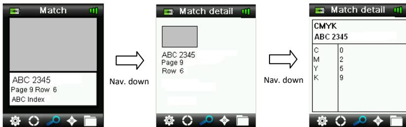
**Note:** The additional match details that display depend on the fan deck used.
