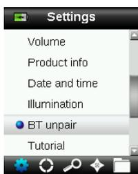
2. Press the **Enter** button to unpair the device. An Unpair succeeded screen appears.
