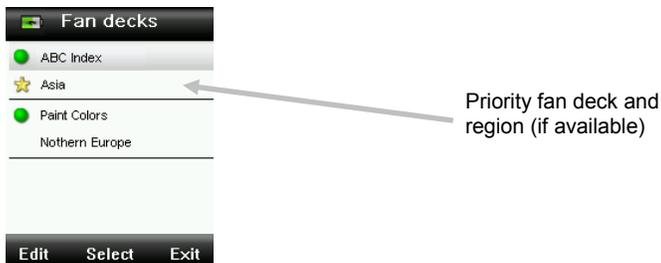
4. Select the fan deck settings option from the list by pressing the up and down sides of the **Navigation** control.
