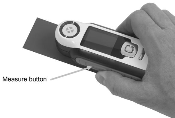
Horizontal, vertical, and angled orientations are acceptable as long as the instrument makes good contact with the sample.
