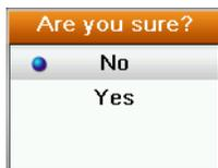
3. Highlighting **Yes** on the screen and press the **Enter** button. The instrument is now reset and all stored records are deleted.
