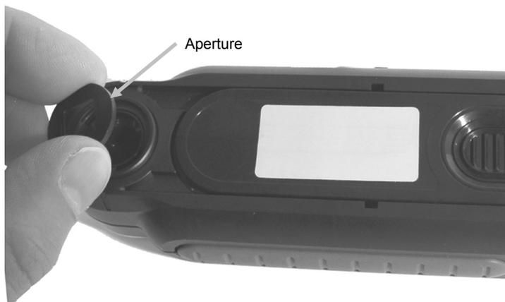
3. Blow short bursts of clean, dry air into the optics port. This should remove any accumulated debris from the optics.
