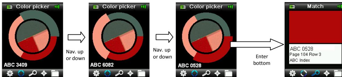
4. Select the desired color by pressing **Enter** to display details of the match.
