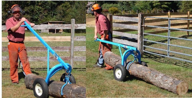
**Note:** when using the arch in a brushy area where the wheels won't roll; **pump** the log out, by setting the tongs, bringing the wheels toward you and as you lift the log, the log will travel toward you about one foot, drop the log and repeat.
