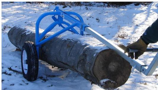
The 5' handle gives you plenty of leverage to easily lift logs weighing up to 1800 lbs with just a quick push on the handle from your shoulders to your waist.
