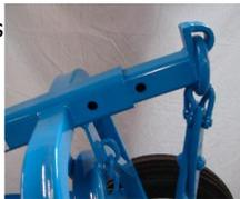
down position for smaller diameter logs
