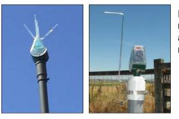
Either install a bird deterrent on top of the node (available from your supplier) or install a bird perch higher and facing away from the node.
