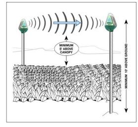
the gaps. There can be three End Nodes per Relay Node, not to exceed 20 total nodes per Base.
