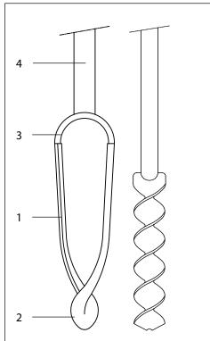
Edelman auger combination type (left) and spiral auger (right)
