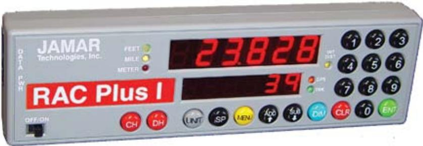
**Fig. 1.1 — RAC Plus I Distance Measuring Instrument**
