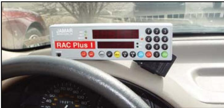
Fig. 2.9 - 'L' Bracket on Curved Dashboard
