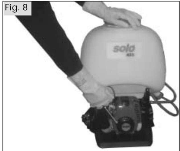
Place the high pressure sprayer on the ground. Ensure the sprayer and the person to start the machine are in a steady position. Ensure the trigger handle on the spray wand is closed and not open for continuous spraying.
