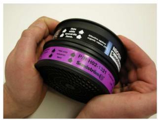
Press the filter/cartridge together so that the arrows on the particulate filter point towards the chemical cartridge.
