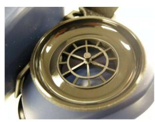
Check and replace worn or damaged parts. Pay special attention to the exhalation membranes. Making sure that they are clean and intact is as important as regular filter replacement.
