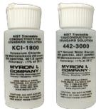
The ULTRAPEN™ PTBT1 uses the following solutions for wet calibration.
