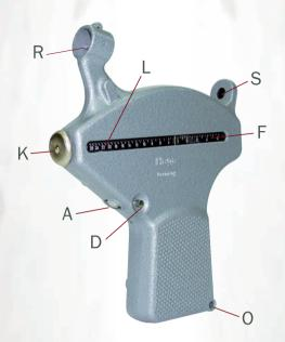
The a.m. height resp. increase values are engraved on a rotating scale bar. The different measuring ranges are adjusted by turning button "K", so that on window "L" on the left side only the adjusted range will appear.
