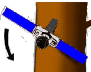
**F.** Turn the auger a quarter of a turn anti-clockwise and keep the extractor knob firmly pressed into the handle. This is very important in order to keep the core intact
