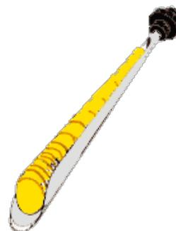
At the start and until the borer engages into the tree a few millimetres, push only moderately hard.
