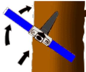
**D.** The borer is now ready for use. When screwing the borer into the tree, consider the following: **Do not use force when starting the penetration.** It may cause damage to your borer and small chips may
