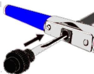
**E.** Insert the extractor into the borer auger (bit) when reaching desired point inside the tree (usually centre of the tree)
