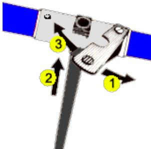
**C.** Turn the lock and insert the auger (bit) in the handle. Then gently turn back the lock until the auger is secured into the handle.
