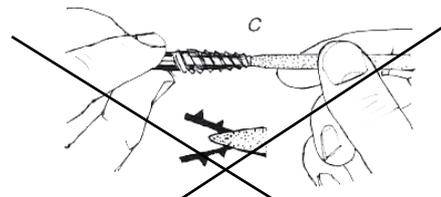
Use the conical stone to smoothen the inside of the borer.
