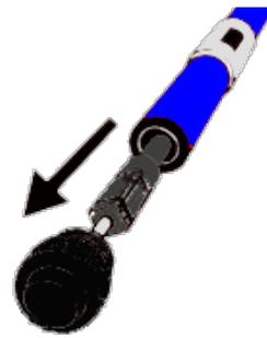
**B.** Remove the borer auger (bit) from the handle along with the extractor
