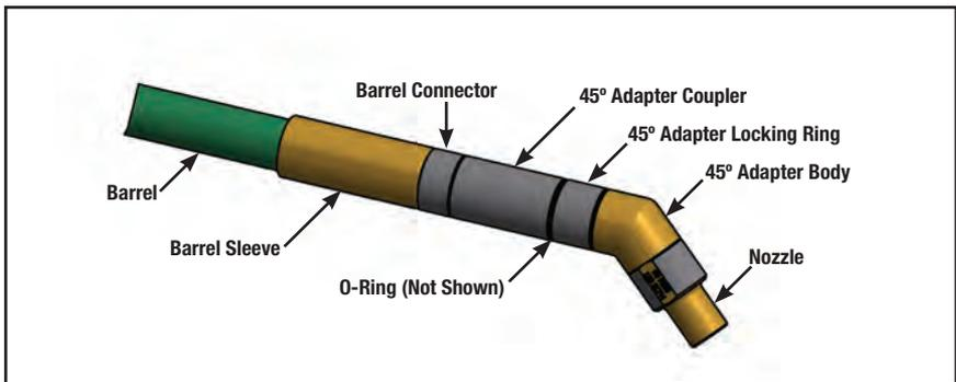
**CAUTION:** When using the 45° adapter, compressed air exiting the nozzle will force the tip of the tool away from the direction the nozzle is aimed. To prevent this from occurring, the operator should place the free hand at least midway down the barrel. Grip the barrel tightly to brace the tool against the force produced by the exiting compressed air.
