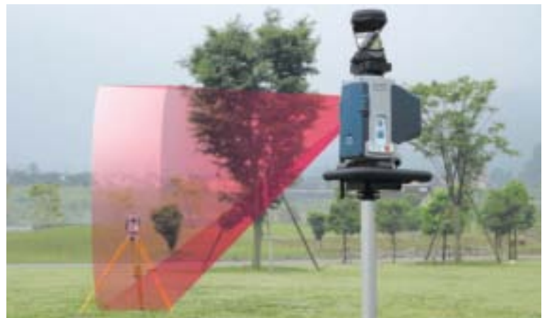
* Red fan beam is for explanation purposes only. The actual search beam is an eye-safe Class 1 invisible laser.
