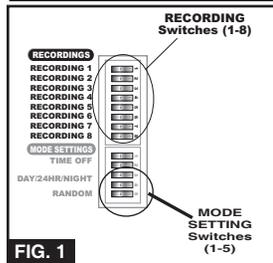
To program your BirdXPeller PRO unit you will need a small screwdriver, toothpick, or other pointed, rigid object to move the switches in the switch array (see FIG. 1). The switch arrays are the switch banks
