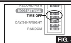
To set the Time-Off period (or delay interval), use the following settings on switches 1 and 2 in the Mode Function Settings.
