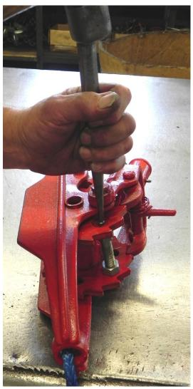
• After rivet is peened down, remove bolt.
