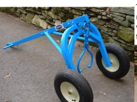
The Junior Arch is a great tool for felling "hung-up" trees, moving logs and bucking firewood. It works on logs 4" to 16" in diameter weighing up to 1000 pounds.
