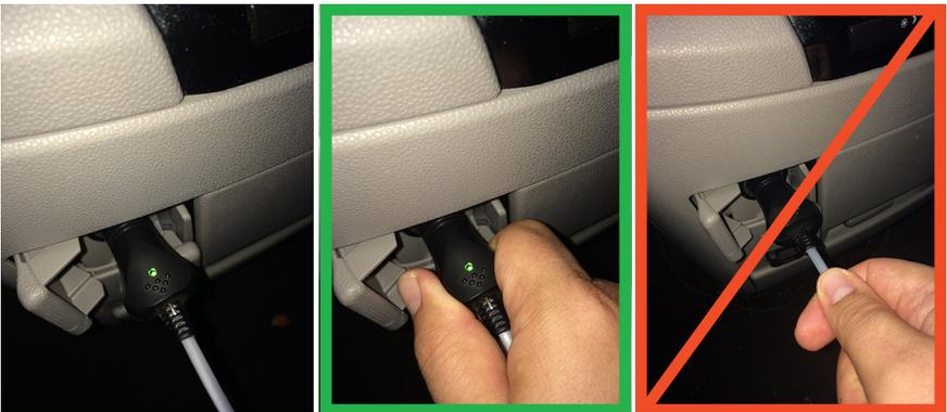
**Fig. 2.6 - Proper Disconnection of Cigarette Lighter Adapter**
