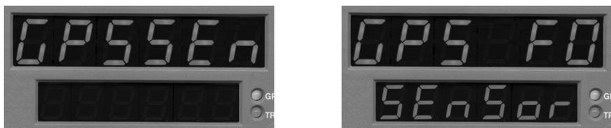
Fig. 3.2 — Internal (GPS) Sensor Mode Start-Up Screens
