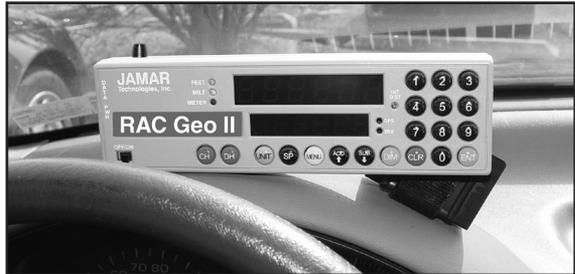
Fig. 2.4 - 'L' Bracket on Curved Dashboard
