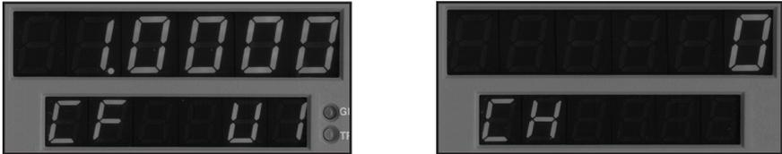
**Fig. 3.5 - Start-up screens for External sensor mode**
