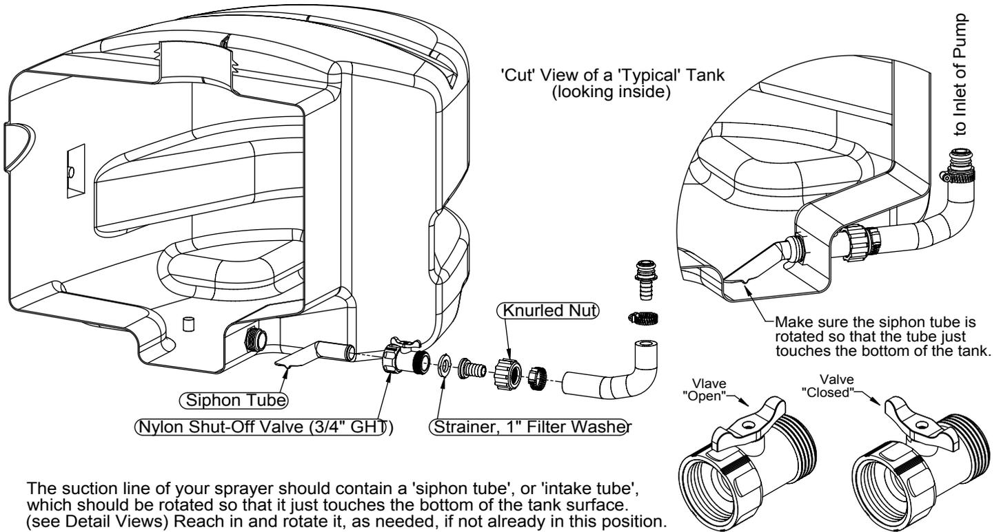
The suction line of your sprayer should contain a 'siphon tube', or 'intake tube', which should be rotated so that it just touches the bottom of the tank surface. (see Detail Views) Reach in and rotate it, as needed, if not already in this position.
