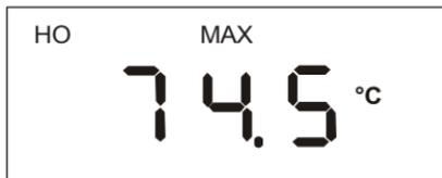
Meter will now continuously display the lowest or highest temperature measured since you entered this mode. It will update the display when new highs or lows are reached.
