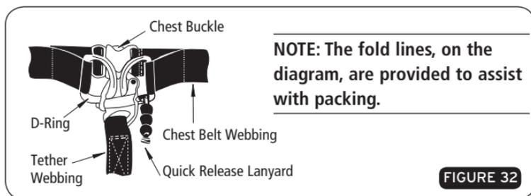
**Warning: Use of a sailing harness to prevent falls overboard presents several risks. In case of capsizing or sinking, the boat may take you down. As such, ensure that any tether used has quick-release under-load hardware. This harness has not been designed for fall arrest, lifting or climbing and should not be relied upon in any of these instances.**
