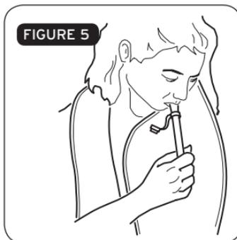
i. To orally inflate the Inflatable PFD, first ensure that each of the zippers (2) are completely opened.
