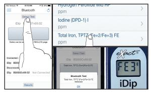
Press (TERO/OD) and the iDip® display reads OPPM indicating the meter is ready to test.
