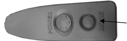
Use the Mode button to select the Laser distance setup (English or Metric). To switch unit in the Laser, select SETUP menu and SET M OR YRD (last menu in SETUP). When in this menu, keep the Mode button pressed down to switch between m or Yard. This unit is only used in the Laser display and has no function in the Vertex display, where metric or feet is used.
