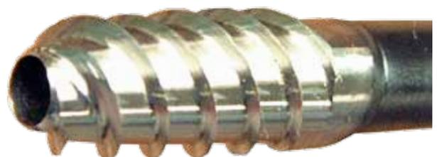
The ease at which a borer penetrates wood depends not only on the threading, but also on type of wood, friction properties and capability of the user.
