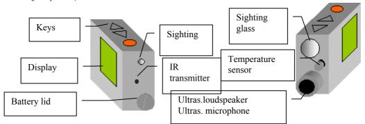
The Vertex III has two (2) arrow-keys and one (1) Enter key marked ON.
