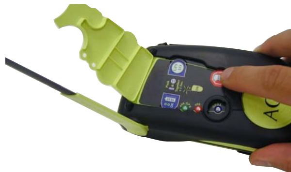
Figure 5 Deactivation Press red OFF button for more than ½ second
