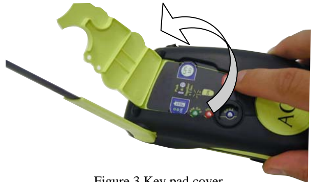
Figure 3 Key pad cover Open the key pad cover for access to Test or activate the beacon
