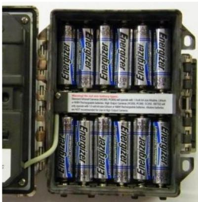
**Warning!** Do not mix battery types! Damage to the camera can result and your warranty will be voided if you mix battery types.
