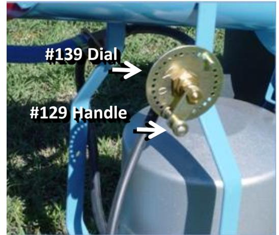
↶ **To increase firing frequency**, turn handle (#129) counter-clockwise, in the direction of the arrow on the dial (#139).
