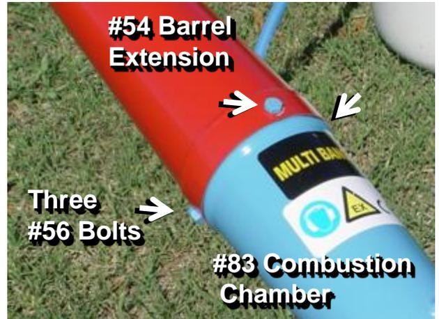
Tighten the three bolts (#56) with a 13 mm wrench.
